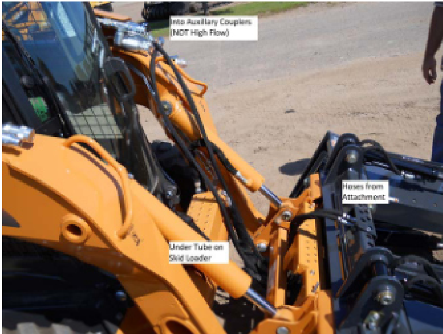
Grapple shown Center Plumb works for Case, John Deere, New Holland, Mustang, Takeuchi, and Gehl skid loaders.
